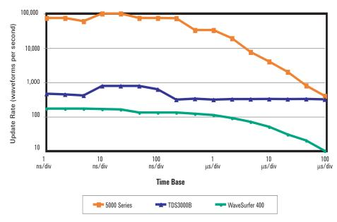
Figure 5. Update rates of popular oscilloscopes using their default real-time time acquisition mode
